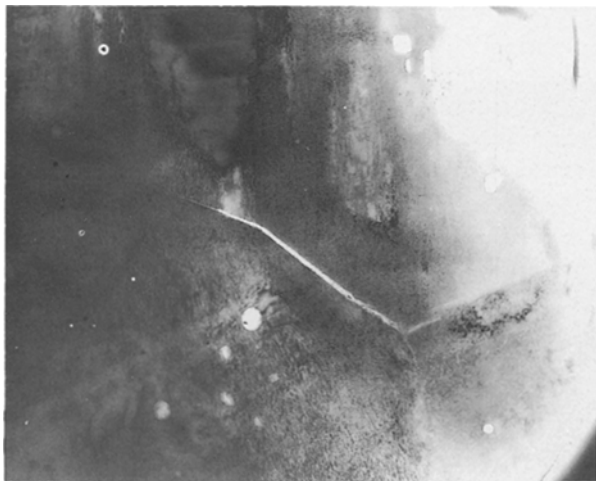
Figure 12 TEM microstructure of Sample b (reacted at 900 °C/24 h and sintered at 1000 °C/8 h) showing some holes inside grains (as indicated by arrows) possibly due to some precipitates dropping out of the matrix during TEM specimen preparation.
